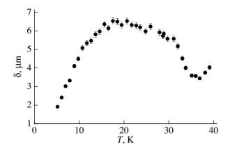
Fig. 9. Temperature dependence of the average size of magnetic inhomogeneities under cooling in a zero field.
