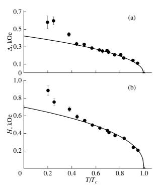
**Fig. 6.** Temperature dependences of (a) the variance  $\Delta$  of static fields and (b) the average field *H*. The curves are fitting of the experimental data using the relation  $H \sim H_{\text{max}}(1 - T/T_c)^{\beta}$ , where  $\beta = 0.40 \pm 0.02$ , which corresponds to the model of a Heisenberg-type 3*d* magnet.
