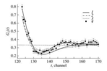
**Fig. 5.** Muon spin relaxation function: (1) processing within the CFM model with  $\chi^2 = 1.02$ , (2) processing within the ASM model with  $\chi^2 = 2.26$ , (3) processing within the SG model with  $\chi^2 = 2.6$ , and (4) experimental points obtained at T = 28 K in a field  $H_{\text{ext}} = 0$ . One channel on the time axis corresponds to 5 ns.
