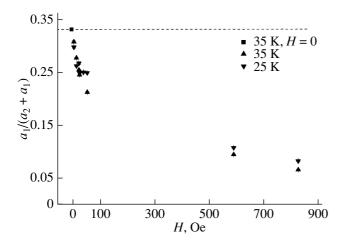
**Fig. 12.** Dependence of the degree of anisotropy on the external field applied to the sample.
