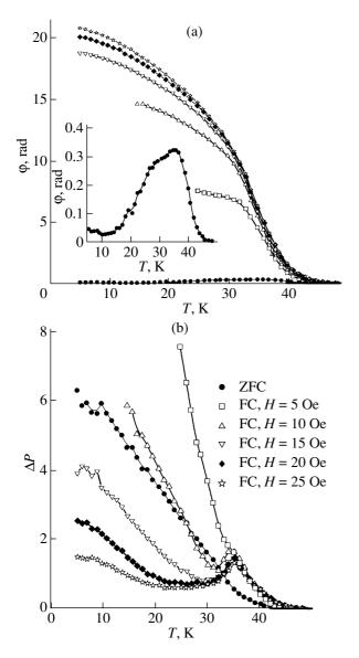
**Fig. 1.** Temperature dependences of (a) the rotation angle  $\varphi$  and (b) depolarization  $\Delta P$ .
