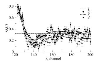
**Fig. 10.** Comparison of relaxation functions: (1) the description of (2) experimental points obtained in an external field  $H_{\text{ext}} = 0$  at T = 35 K within the CFM model and (3) the description (using the function  $G_s(t) = G_s(t) = a_1 e^{-\lambda t} + a_2 \cos(\Omega t) e^{-\lambda t}$ , where  $a_s = a_1 + a_2$ ) of (4) experimental points obtained in an external magnetic field  $H_{\perp \text{ext}} = 28$  Oe at T = 35 K. One channel on the time axis *t* corresponds to 5 ns.
