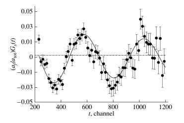
**Fig. 3.** Muon spin precession in an external magnetic field  $H_{\perp ext} = 32.6$  Oe at T = 35 K;  $a_{tot} = 0.2893(32)$ ,  $a_f = 0.0090(8)$ , and  $\lambda_f = 0.092(4) \,\mu s^{-1}$ . On the time axis *t*, one channel corresponds to 5 ns.
