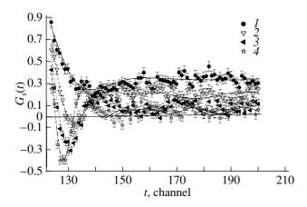
**Fig. 11.** Relaxation functions  $G_s(t)$  for various values of the external magnetic field  $H_{\perp ext}$ : (1) 0, (2) 410.0(2), (3) 590.0(2), and (4) 824.0(2) Oe at 35 K. One channel on the time axis t corresponds to 5 ns.
