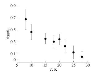
**Fig. 8.** Temperature dependence of the fraction of the spinglass contribution to the depolarization of a muon ensemble.
