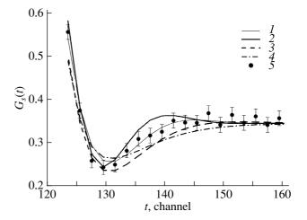
**Fig. 7.** Muon spin relaxation function: (1) the description by the sum of two functions CFM + SG with  $\chi^2 = 1.0$ , (2) processing within the CFM model with  $\chi^2 = 1.23$ , (3) processing within the ASM model with  $\chi^2 = 1.58$ , (4) processing within the SG model with  $\chi^2 = 1.85$ , and (5) experimental points obtained at T = 15 K in a zero external field. One channel on the time axis *t* corresponds to 5 ns.
