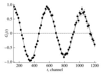
**Fig. 2.** Muon spin precession in an external magnetic field  $H_{\perp ext} = 32.7$  Oe at T = 61 K;  $a_{tot} = a_s + a_f = 0.2893(32)$ ;  $\lambda = 0.077(5) \ \mu s^{-1}$ . On the horizontal axis, one channel corresponds to 5 ns.
